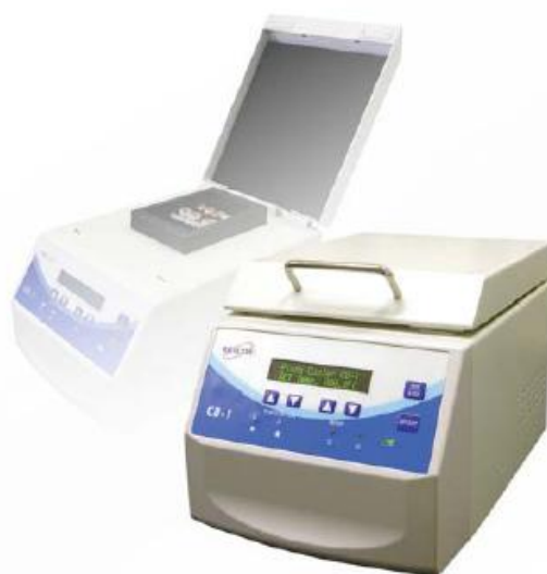
Figure 1: Wealtec's CB-1 Block Cooler. With a temperature range from 0 to 70°, CB-1 covers a wide range of incubation applications within fields of molecular biology. CB-1 has 9 pre-set temperatures and customised temperature setting is extremely easy. An insulated lid and exact temperature control makes CB-1 perfect for e.g. restriction digestion applications.
